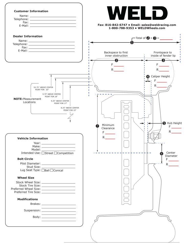
NOTE: MEASUREMENTS SHOULD BE TAKEN WITH SUSPENSION AT NORMAL RIDE HEIGHT
